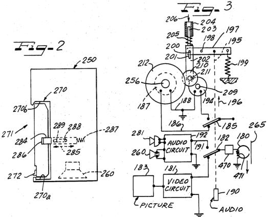
TRANSDUCER MACHINE FOR SLIDEABLE RECEPTION OF AND AUTOMATIC ELECTRIC CIRCUIT CONNECTION WITH A HAND HELD TYPE SELF-CONTAINED TAPE RECORDER
