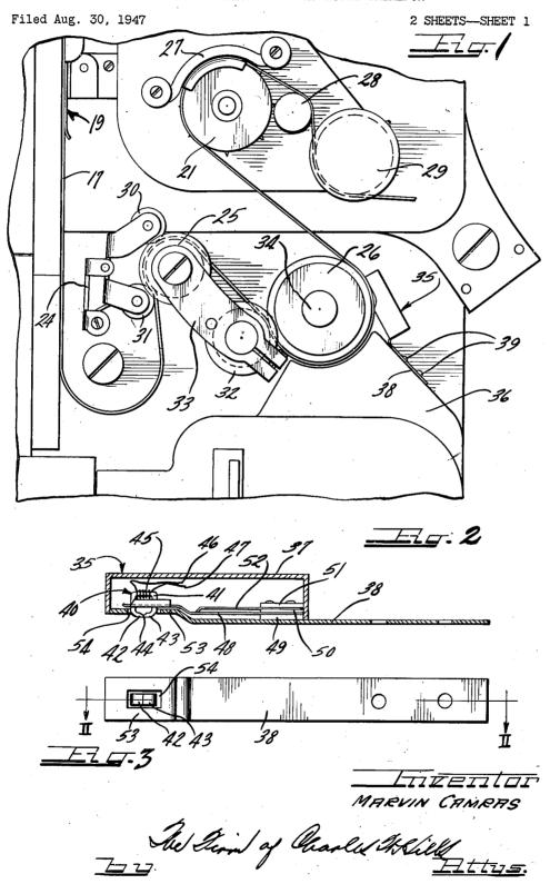
MAGNETIC PICKUP HEAD AND MOUNT THEREFOR
