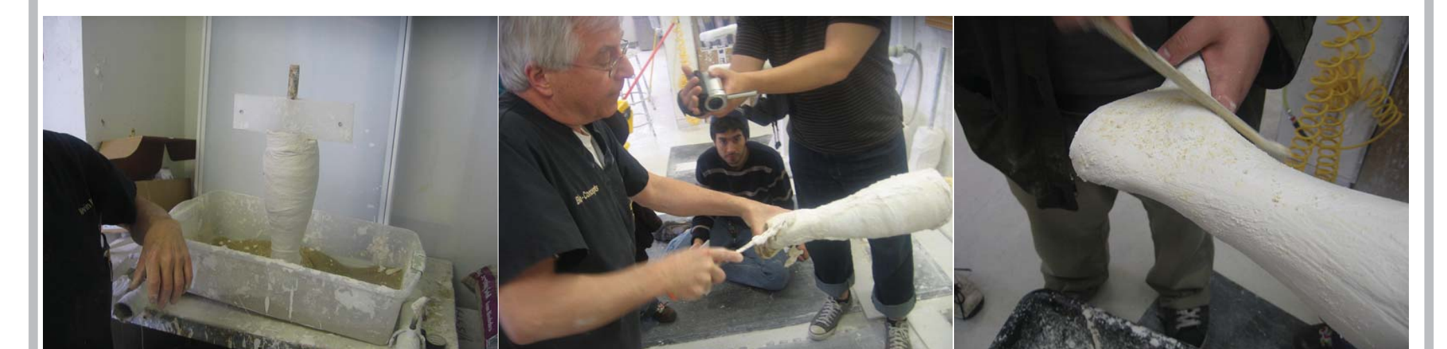
Casting positive mold of the leg in plaster and reshaping the plaster cast
