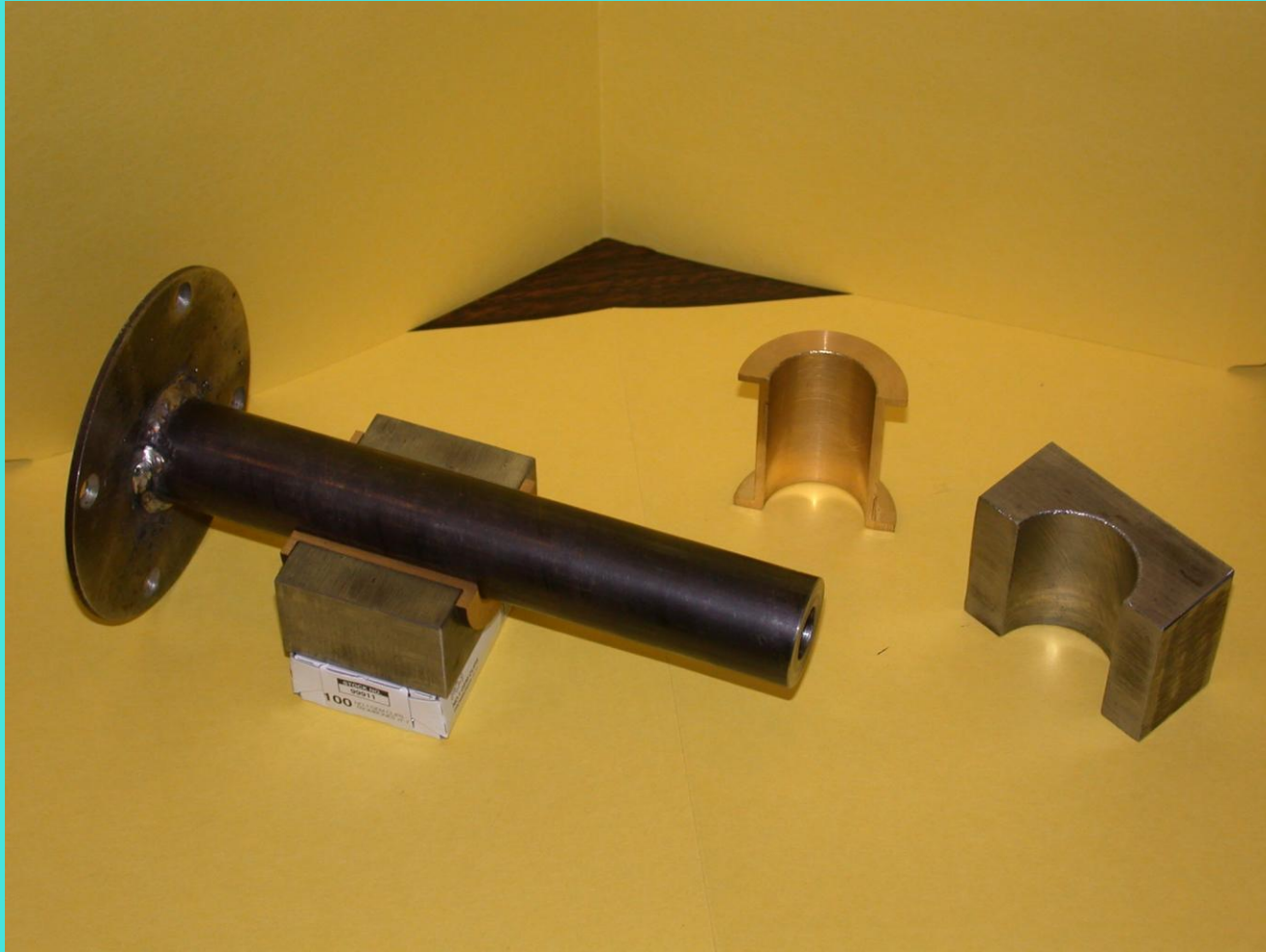
First iteration of hollow axle from this semester
