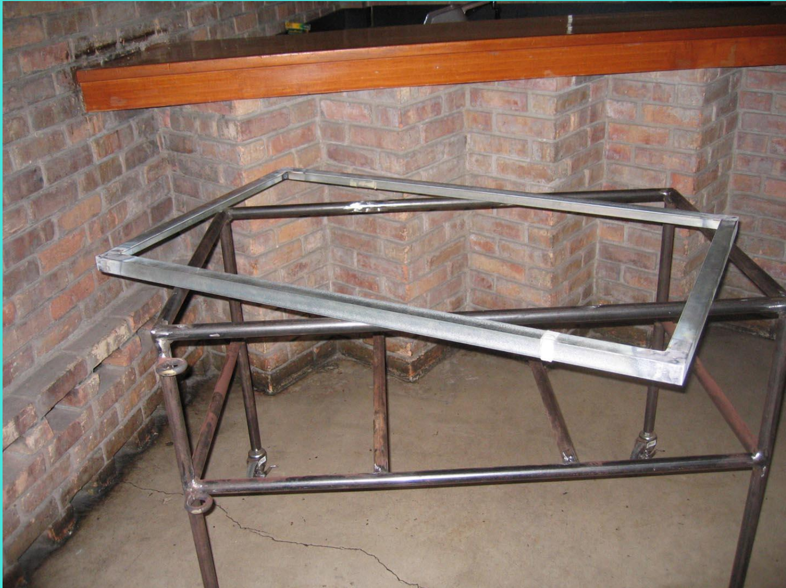
Stand (with casters) and drum support frame developed this semester
