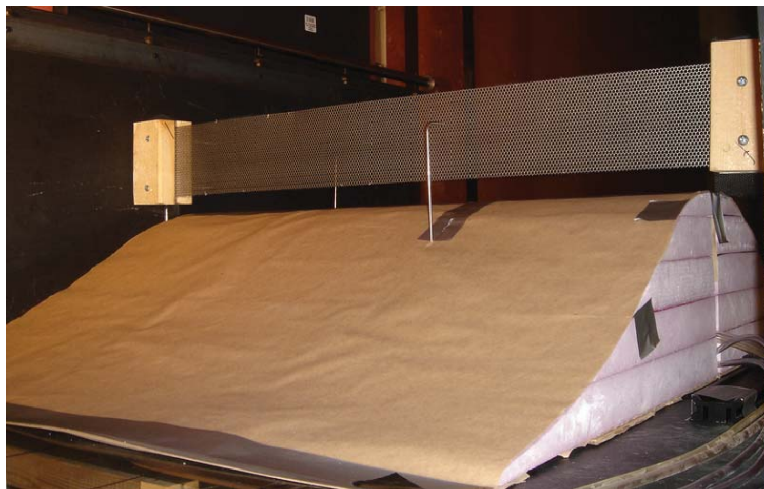
Final constructed shape with mesh attached mounted in the wind tunnel for testing. Located in the center of the picture is one of many pitot tubes used for data collection.
