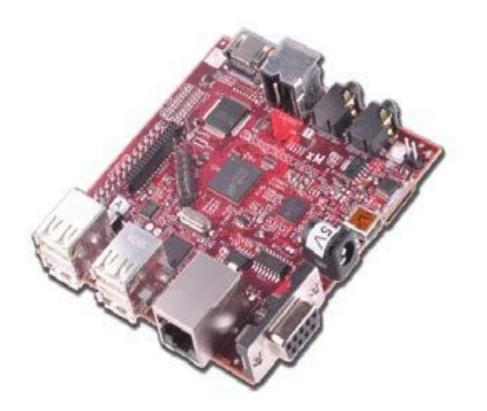
$3.25^{"} \times 3.25^{"}$ 113 grams 4 USB 2.0 ports 10/100 ethernet port 1-GHz ARM® processor 512 MB of RAM
