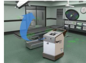
Phase one: Dehumidification Conditioned (dried) air is injected into the enclosure and moisture is removed.
