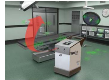
Phase one: Dehumidification Conditioned (dried) air is injected into the enclosure and moisture is removed.
