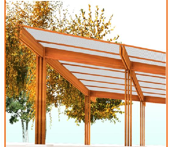
Roof structure is detached from the wall structure for independent movement from the wall structure during seismic activity
