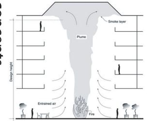
In large volumes such as atriums the exhaust method is often used. This process removes the smoky air from the top of the space, while replacing it with clean air from the base. The clean (make up) air can be mechanically or passively added to the space depending on the specific requirements outlined in the job.
