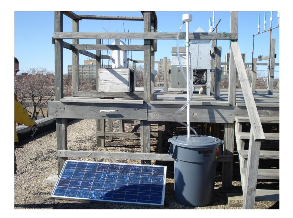
The test pump used with the DC inverter was then tested with a solar panel. The setup shown above has the solar panel connected to the pump which is submersed in the garbage can full of water. The water in pumped up through the PVC pipe to the cup at the top and returns to the garbage can via the clear tubing. This system allowed for continuous testing without fear of burning the pump out if the water supply ran dry.
