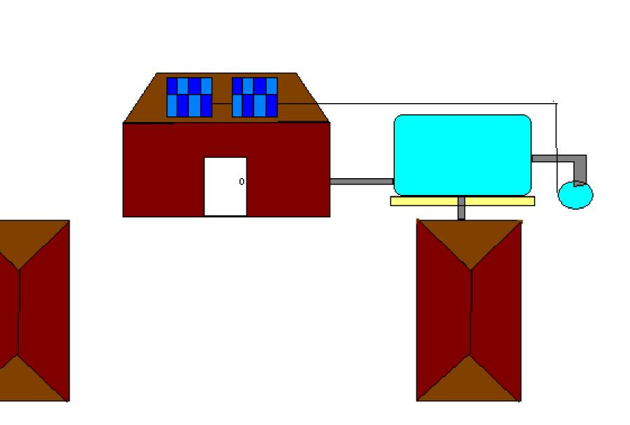
Phase one of the Kankakee implementation will focus on the oumping system, while not incorporating distribution. A well will be dug, and Solar panels will be installed on the roof, which will power the pump inside the well. Water will be pumped into a torage tank which will be at ground level on top of a concrete lab. The performance of the system can then be analyzed and iny necessary changes can be made. During this phase, water nust be obtained from a faucet on the storage tank outside.
