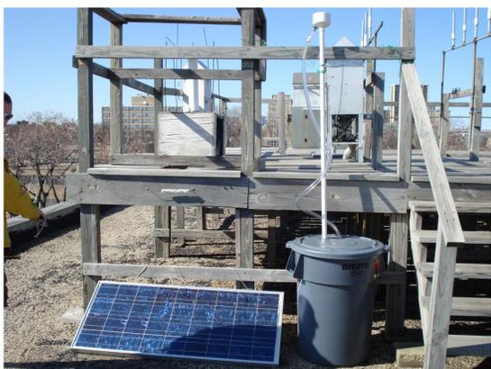
The test pump used with the DC inverter was then tested with a solar panel. The setup shown above has the solar panel connected to the pump which is submersed in the garbage can full of water. The water is pumped up through the PVC pipe to the cup at the top and returns to the garbage can via the clear tubing. This system allowed for continuous testing without fear of burning the pump out if the water supply ran dry.
