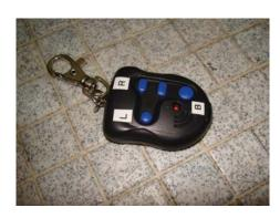
RF kit is used to transmit signal to activate left and right vibration motors that will be attached on the swimmer
