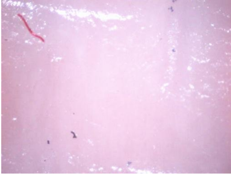
Fig. 2: Surface of porcine skin after submersion in green dyed water and application of vacuum for a period of 1.5 hours.
