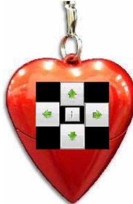
Unit back showing buttons to control who receives the message, message content, sending messages, and on/off.
