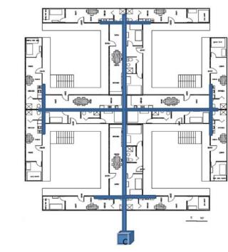
tank, which is placed adjacent to the building such that the required water pressure is achieved via gravity and buoyancy, essentially a thermosiphon water system. About 65-95% of water heating will come from the sun and the rest will be supplied via an electrical heating element within the tank that will function as a back-up heating source. Further work will include to create detailed drawings that address all connections and set-up
