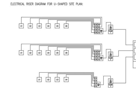
quence meter stacks. These stacks give us the ability to meter the power usage per unit as opposed to per site, which ultimately causes less problems with billing issues in the future. These circuit transformers (three per U-plan and four per Cross-plan) are then wired to the main circuit breaker which is supplied with the main power service. The power distribution lines were mapped out for each plan specifying service sizes, wire sizes, and wiring configurations.
