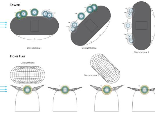
WIND SPEED INCREASE FACTOR WAS DETERMINED BY CALCULATING THE RATIO OF THE WIND VELOCITY AT THE CONTROL POINT WITH THE VELOCITY AT THE TURBINE LOCATION.
