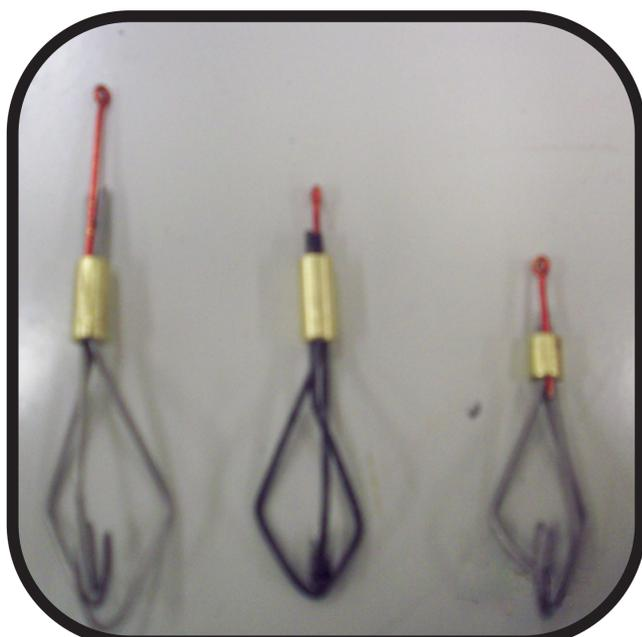
**7a** The two pieces of wire are joined together using a crimped piece of copper
