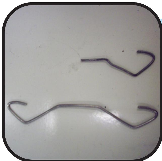
**4** Using a template, the wire is hand bent into the profile of the Delta Hook
