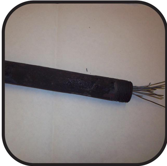
**1** Wire and charcoal are placed into a pipe and sealed airtight
