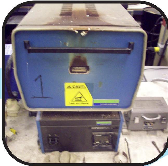
**2** The pipes are placed into an oven to allow the wire to normalize
