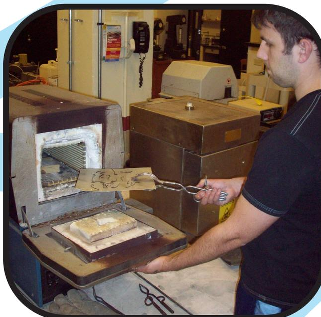
**5** The bent hooks are placed into an oven to be heat treated and then again to be tempered
