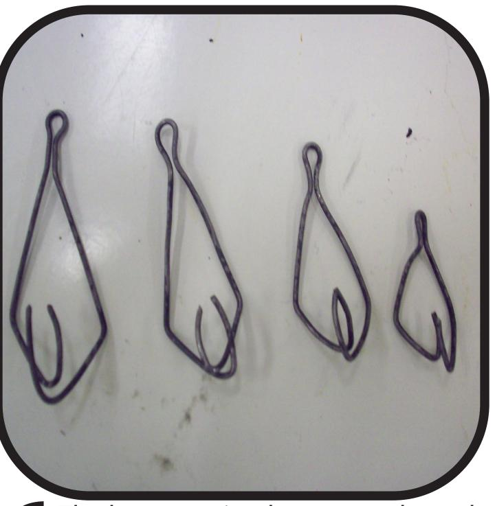
Using a template, the wire is hand bent into the profile of the Delta Hook
