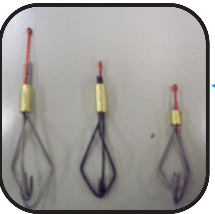
The two pieces of wire are joined together using a crimped piece of copper
