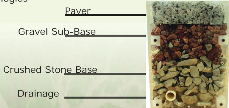
This system takes a slightly different take on permeable paving. Precipitation travels through three layers and is lead into a drainage pipe. This pipe then directs the water to a new desired location, also allowing for stormwater collection.
