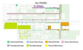
The use of permeable pavements helps reduce the run off volume experienced during storming. A growing issue on campus is the collection of water on sidewalks and other paths. This map illustrates the types of pavement and where they would be most effective.
