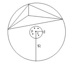
Diagram 4 : Point insertion if the case is a sliver
