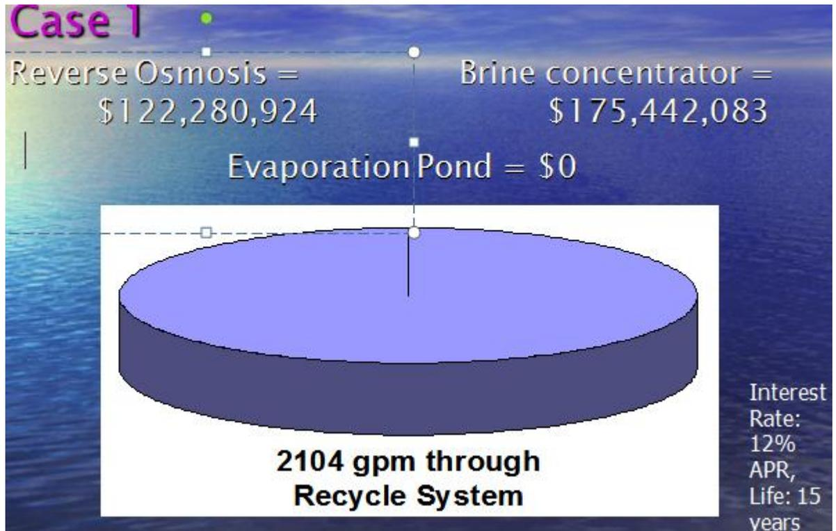
The second case requires the use of the existing evaporation pond at the power plant in addition to the use of reverse osmosis and a brine concentration unit. The excess of 1488 gallons per minute that is unable to fit in the existing evaporation pond would be purified for reuse within the plant.
