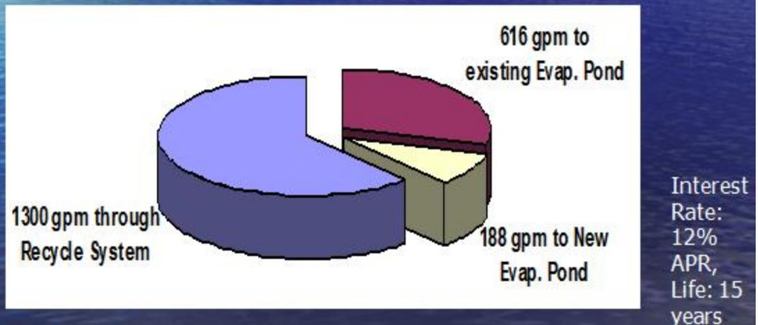
The final case is an arbitrary one. This case involves 1300 gallons per minute being recycled and the rest being placed into an additional evaporation pond. This value for the amount of water recycled was chosen as an intermediate value between the extreme of recycling all the waste water and recycling the bare minimum amount of water necessary for the power plant to function.
