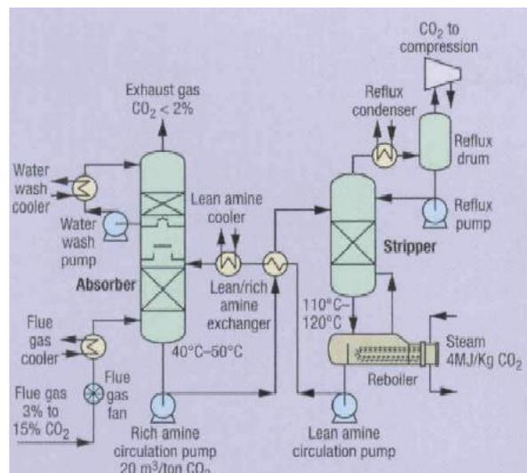
**Figure 3: Diagram of an amine removal system**
