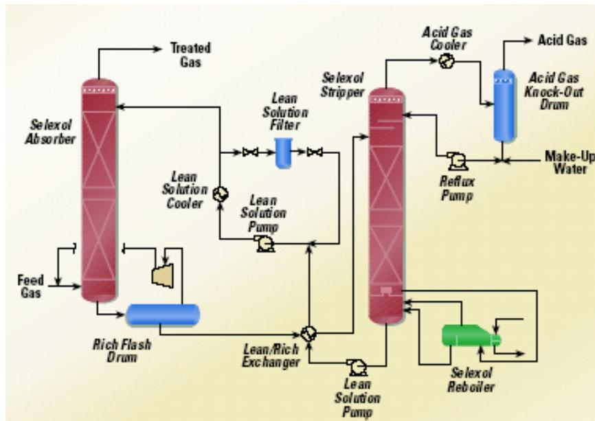
Figure 5: Diagram of the Selexol Process
