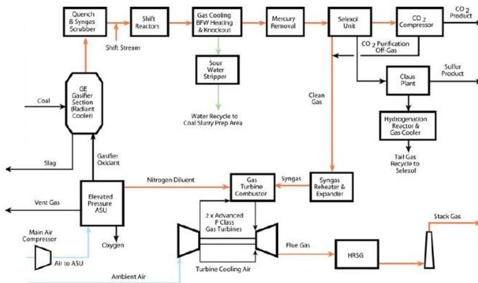
Figure 10: Diagram of GE's IGCC Design
