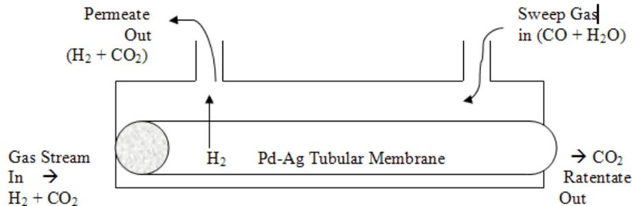
Figure 6: Diagram of Counter-flow Membrane Reactor
