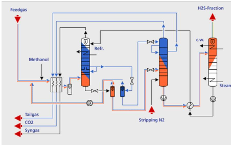
Figure 4: Diagram of a Rectisol System
