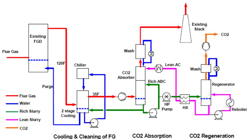
Figure 7: Alstom's CO<sub>2</sub> removal system
