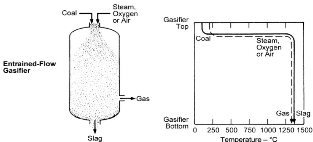
Figure 11: Entrained-Flow Gasifier (GE, ConocoPhillips, Shell, Siemens, MHI)
