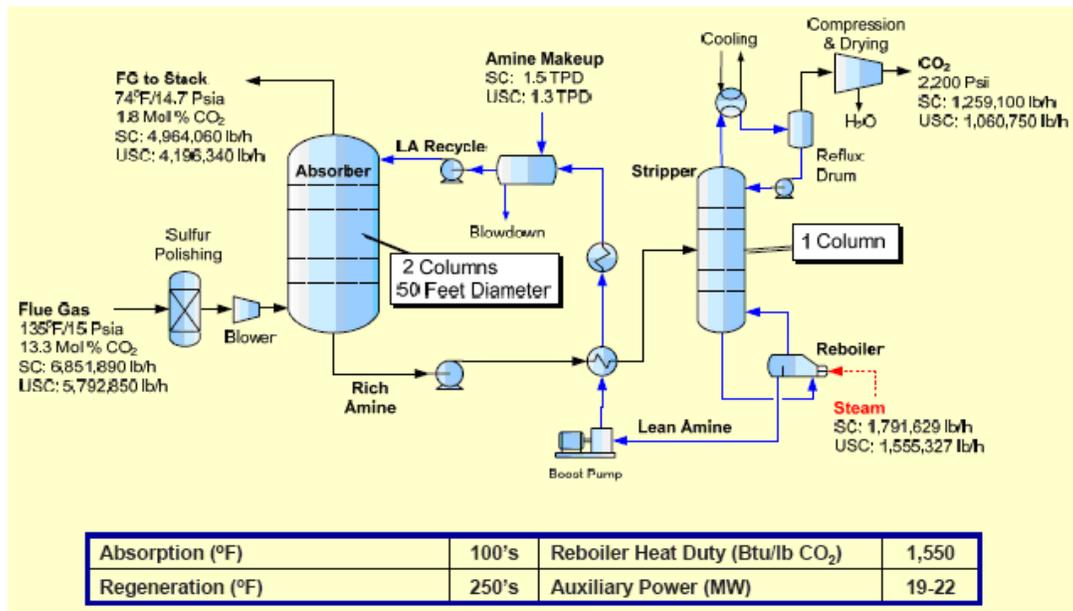
Figure 8: Fluor's Ecoamine CO<sub>2</sub> Removal Process
