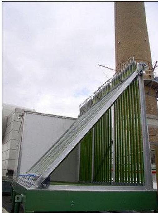
**Figure 2** shows the set-up of the bioreactors design for algae growth. This picture is from a study by GreenFuel Technologies in Cambridge, MA. They field tested a closed system that uses the CO<sub>2</sub> in power plant flue gases to feed algae, akin to the design we would be using.
