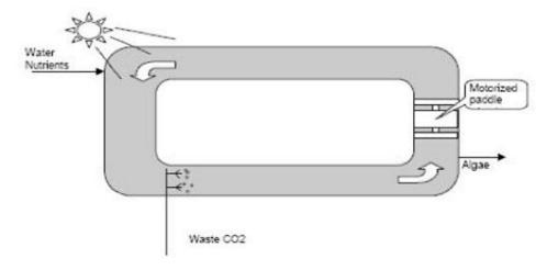
**Figure 1** shows the set-up of a raceway style algae growth design with the water flowing in a counterclockwise direction around some sort of barrier in the middle. The flue gas is pumped into the algae flow and mixed in to provide turbulence and carbon dioxide.
