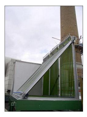
**Figure 2** shows the set-up of the bioreactors design for algae growth. This picture is from a study by GreenFuel Technologies in Cambridge, MA. They field tested a closed system that uses the  $CO_2$  in power plant flue gases to feed algae, akin to the design we would be using. (http://www.oakhavenpc.org/cultivating\_algae.htm)
