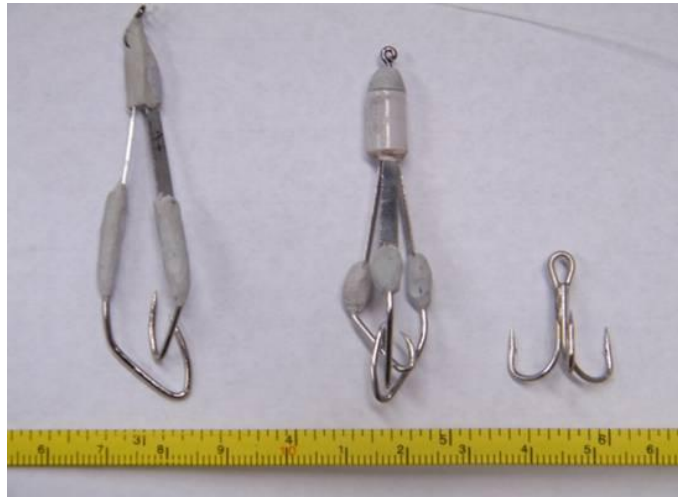
From left to right mock-up E, mock-up F, and the standard treble hook
