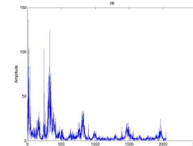
← Here is an FFT chart taken when tested with 8 broken teeth. There is an abnormal spike in data recorded.
