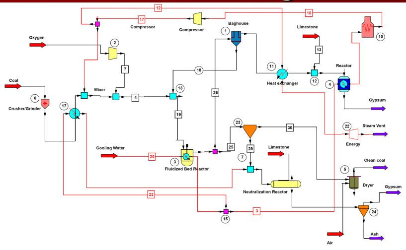
**Diagram 2: Oxydesulfurization Process**
