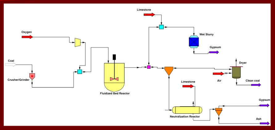
Diagram 3: Simplified Oxydesulfurization Process
