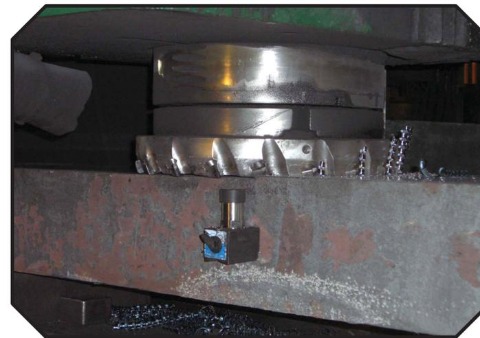
Finkl Mill with Accelerometer Attached underneath
