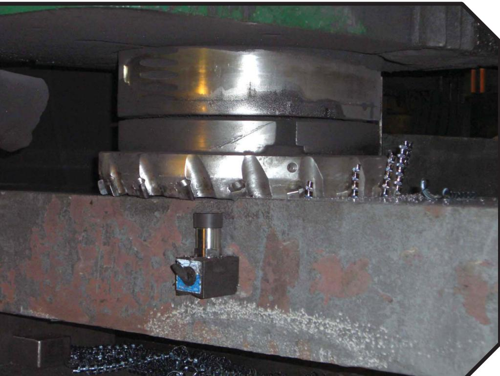
Finkl Mill with Accelerometer Attached underneath
