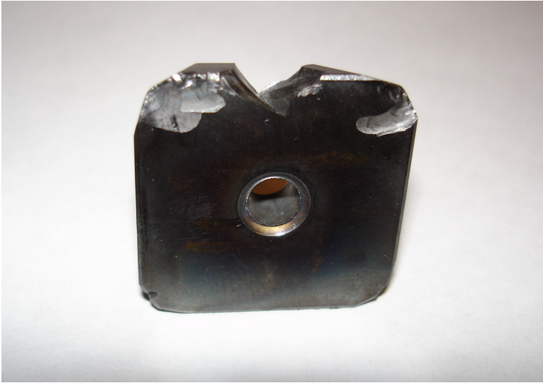
Figure 1. Broken Cutting Insert
