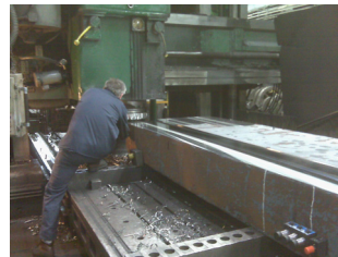
Technician Replacing a Broken Tooth
