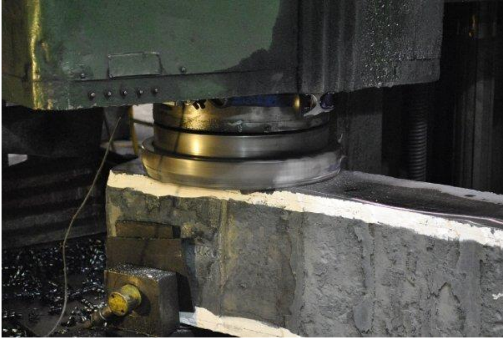
Figure 17 A Finkl & Sons' Vertical Spindle Milling Machine
