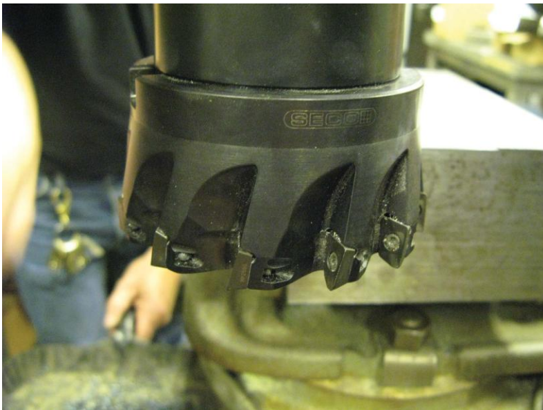
Figure 14 6" diameter milling cutter on IIT's manual milling machine
