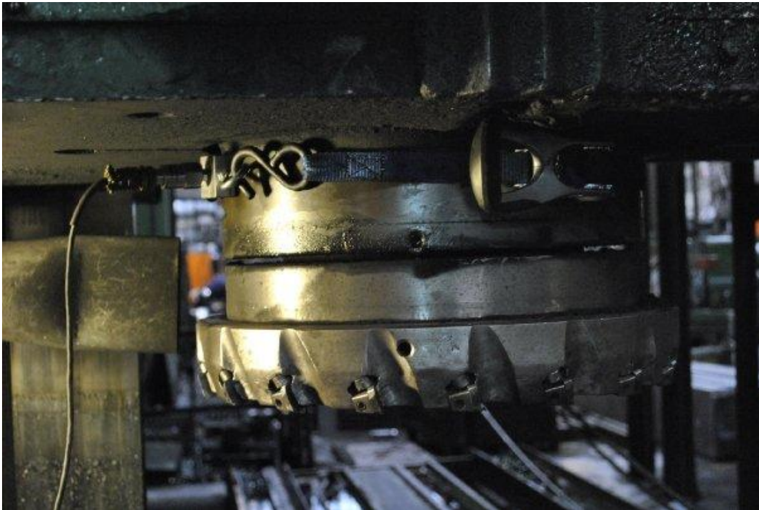
Figure 18 Custom made mounting for accelerometer on A Finkl & Sons' milling machine
