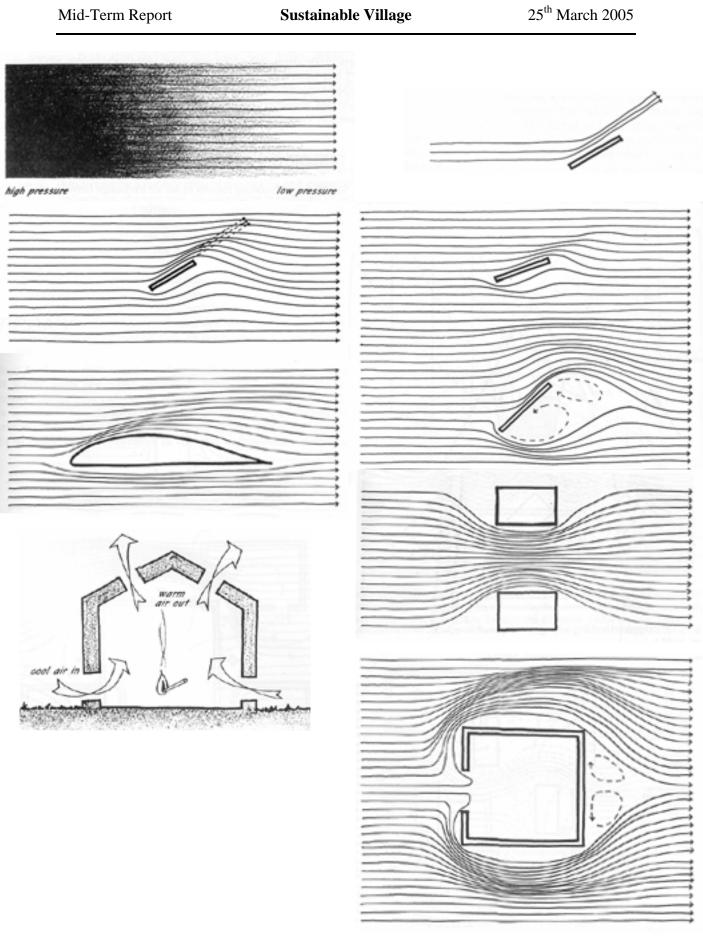
Research conducted at the Texas Engineering Experiment Station in the 1950s developed a guideline for ventilation in buildings and devised these diagrams that embody the principles of passive cooling.
