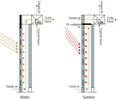
**Figure 1**: PV back air flow is preheated for the house ventilation system in the winter and ventilates the façade in the summer
