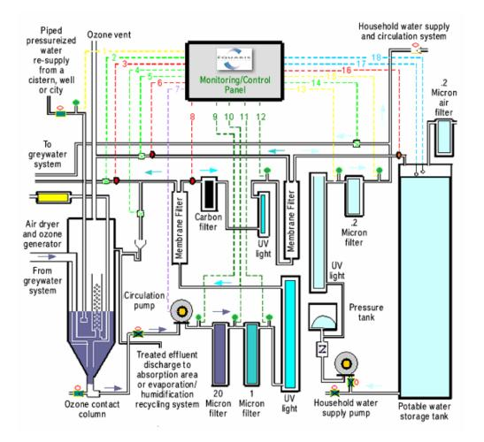
The following graphic shows the schematic layout of the filtration system:
