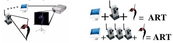
"Simple" in design, these single camera installations usually provide some one on one interaction with the participant. Requiring just a single camera, these projects read the participants' shape and motions. Through custom made programming this input alters the projected image however the artist wants. More complex installations often use multiple camera inputs to produce complex image compositions. In this example, Utterback composes four different views of the participant into one image.
