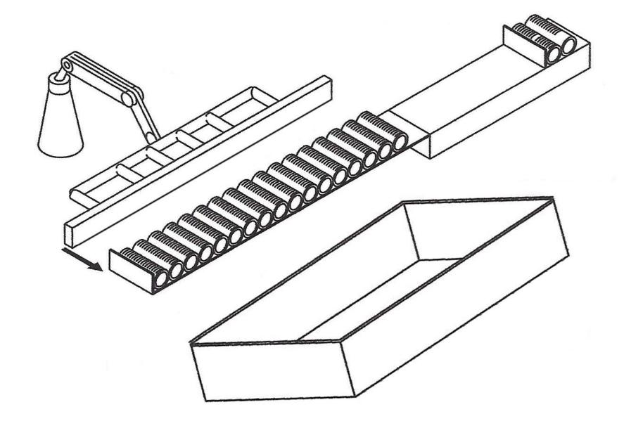
Pins are automatically loaded into standard bins, one full row at a time.
