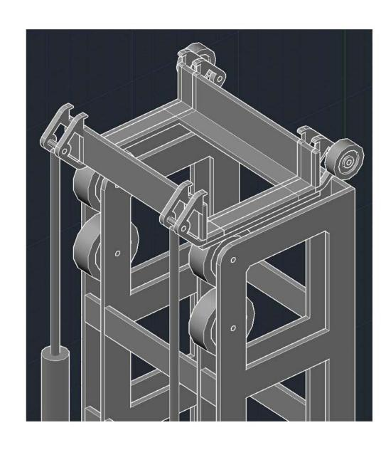
Metal bins are fed to loader by conveyor. Bin is fixed into a grip, lowered and tilted to allow for quick filling using a shelf with pins that are pushed into the bin by a hydraulic press.
