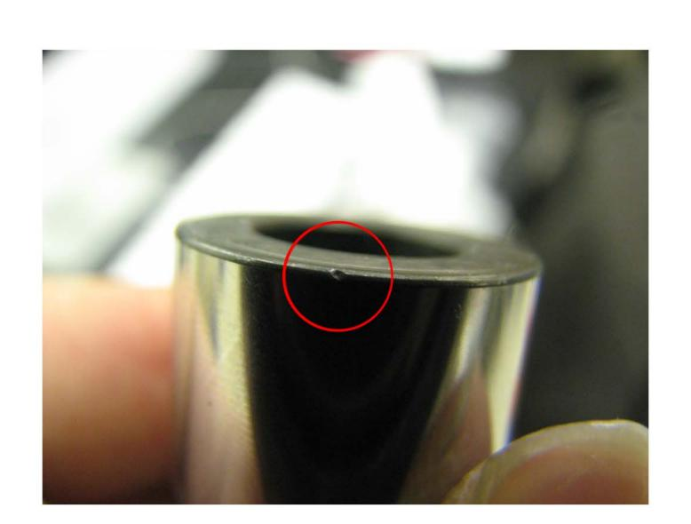
Nicks on outer diameter of pin are unacceptable.
