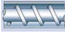
The inner core prevents flooding/overfeeding of the solid material being conveyed. Within the flexible screw conveyor, the gap between the spiral and tube must be less than 1mm, so that the zinc pellets may pass with ease and agglomerations are reduced. A small motor will rotate the flexible screw conveyor.
