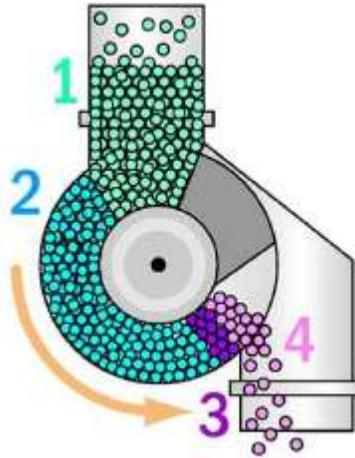
The BSP feeder also allows an easy way of monitoring how much zinc is being dispensed to the car by providing a uniform flow rate of particles.
