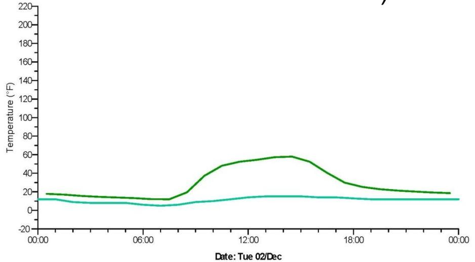
Air temperature: Room 001 (crude\_construction.aps)    Dry-bulb temperature: (ChicagoMidwayTMY.fwt)
