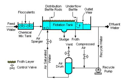
Fig 5.1, Flowchart of DAF Unit in Wastewater Treatment<sup>[6]</sup>
