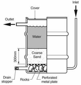
Fig 5.2, Tertiary clarifiers using rapid gravity filtration<sup>[7]</sup>
