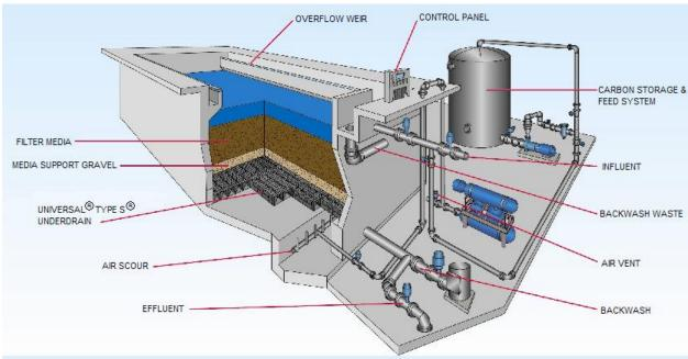
Fig 4.2, Typical Leopold Elimi-NITE System<sup>[5]</sup>
