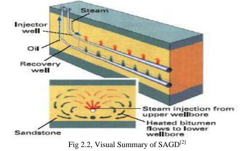
Extraction Method 2: Steam assisted gravity drainage (SAGD)
