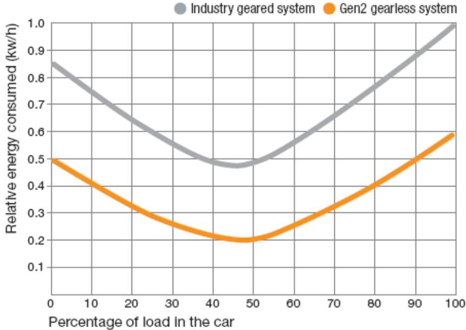
Based on 3500 lb. system at 350 feet per minute and 180 starts per hour.
