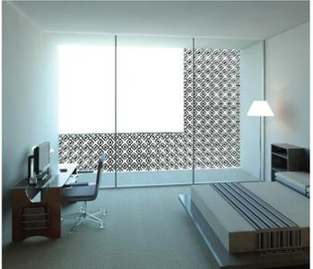
Tower facade has mesh screen that blocks the sunlight and allows natural Ventilation. Window screens are commonly found in traditional Indian architecture.
