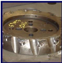
all inserts highly probable. This poor surface finish often forces Finkl to remachine the part to meet customer specifications, and this leads to the loss of significant amounts time and money.
