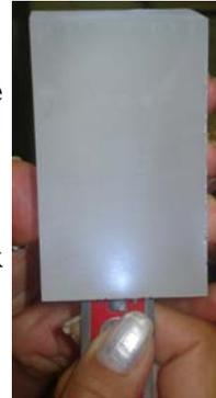
Testing the light transparency of a resin test sample.
