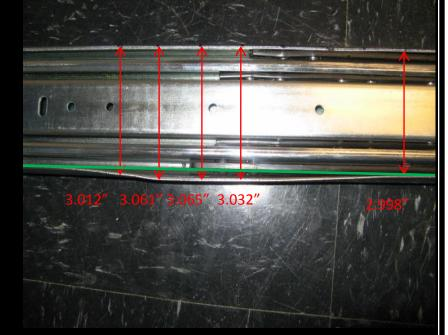
Right slide failed after 680 cycles for 220 lb test
