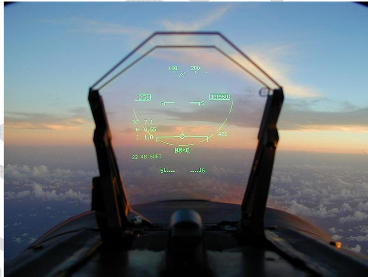
Figure 1. The HUD gives the pilot important flight data while in stable level flight. Some of the data in this particular picture include time, directional heading, aircraft roll, aircraft pitch, aircraft velocity, aircraft angle of attack, altitude. When this aircraft engages a target, more indicators would probably show up on the screen indicating weapon and target information. [20]
