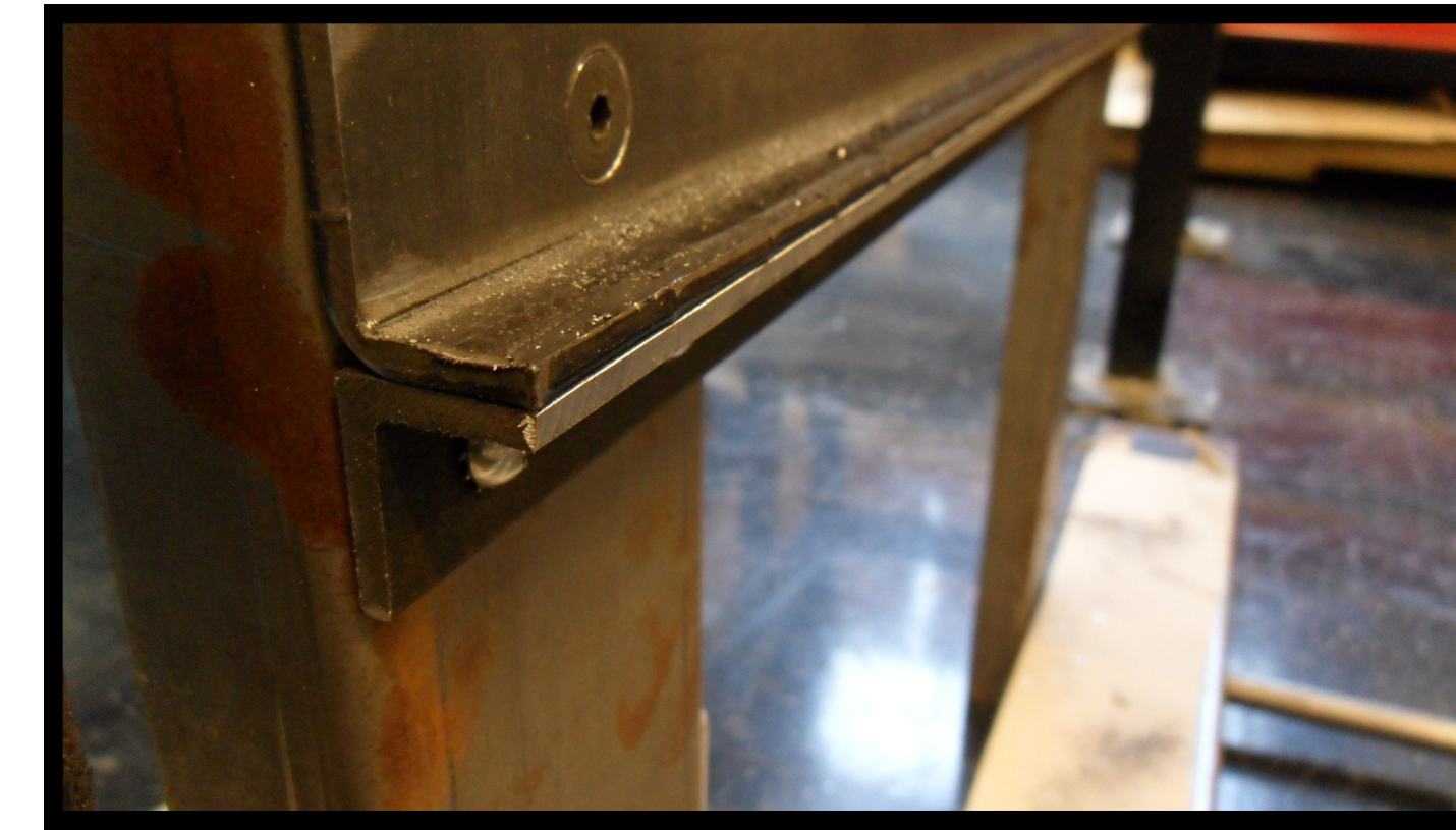
Drawer Slide Shortened (Yellow Line) To Change Point of Contact From Black To Red Arrows, Reducing Moment
