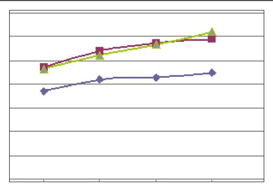
From the results we decided to go with the T3 design, a savonius wind turbine design with three blades. This design provided equal or higher voltage at each resistance level tested.
