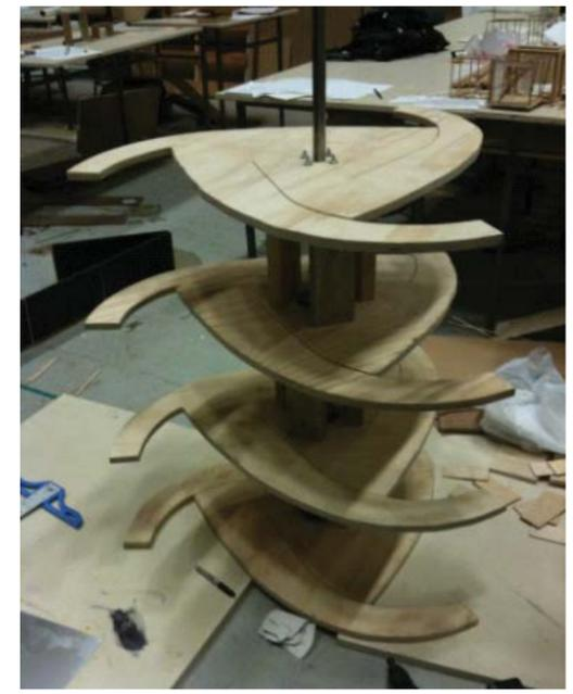
*dry assembly of prototypical wind turbine*
