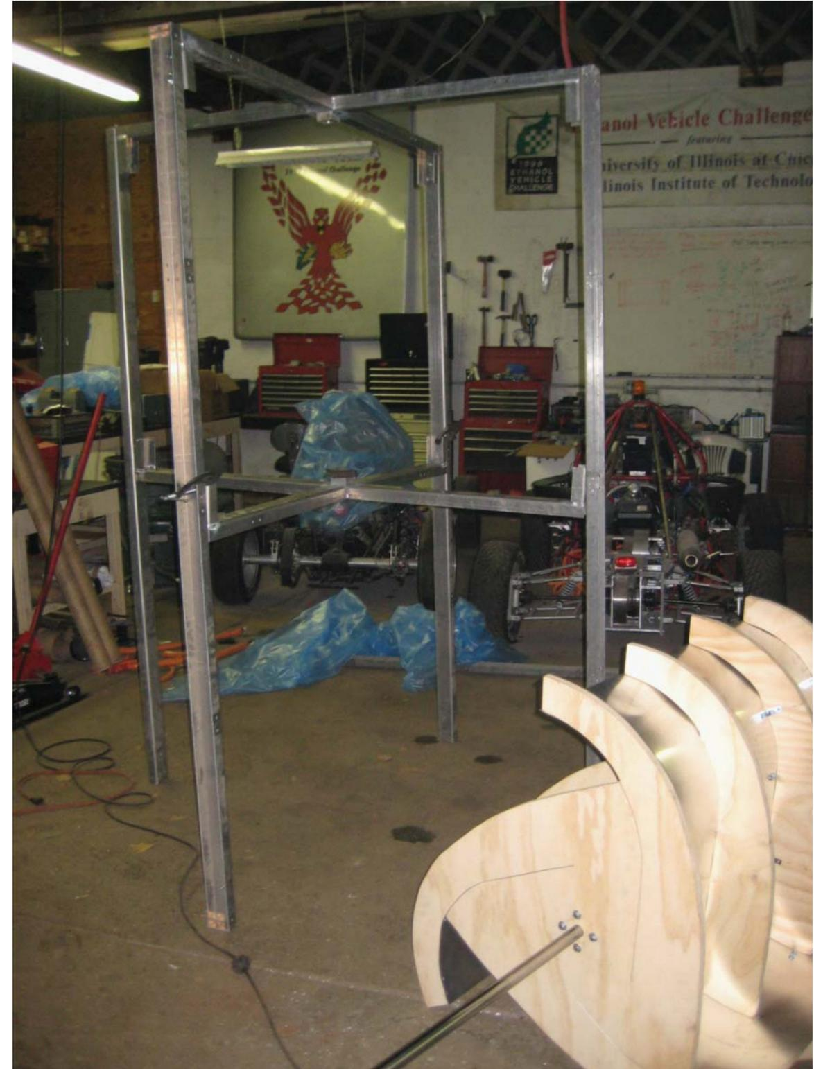
*Savoius-Rotor wind turbine with completed frame*
