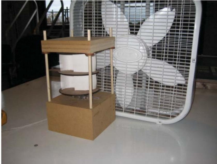
*testing of savoius-rotor triple blade design*
