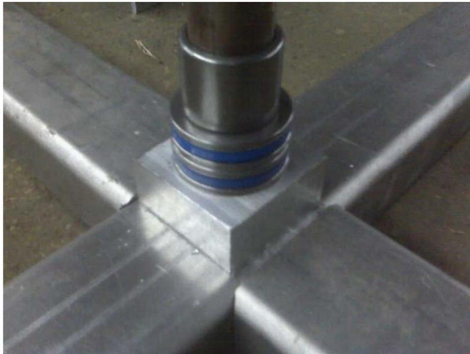
*horizontal cross members with axial support block and ball bearings*
