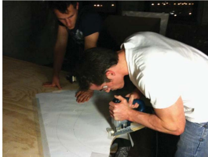
*cutting wind support discs with plotted template*
