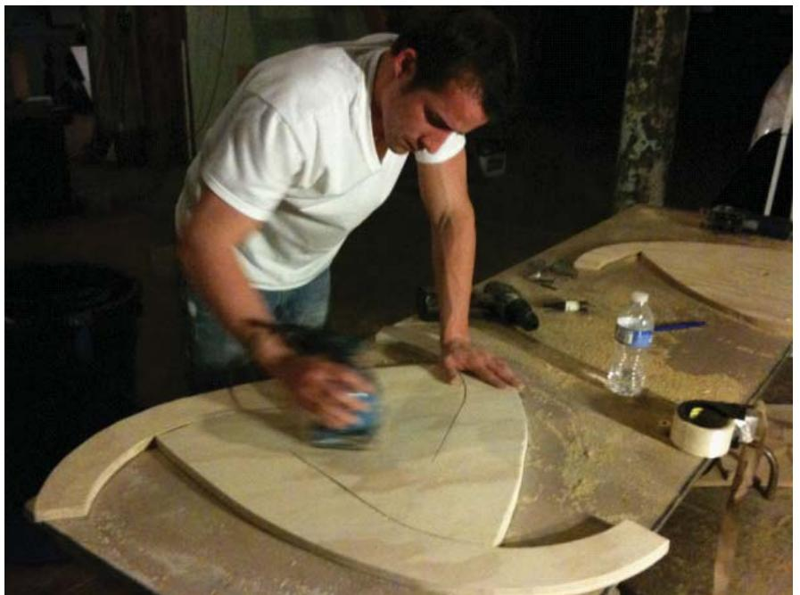
*sanding wind support discs to reduce wind drag*
