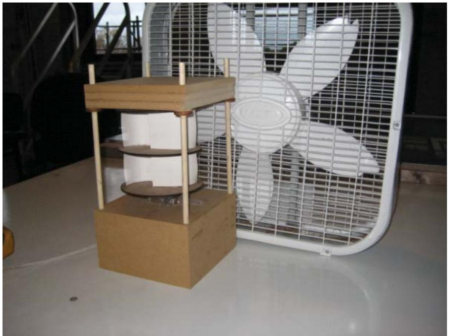
*testing of savoieus-rotor triple blade design*
