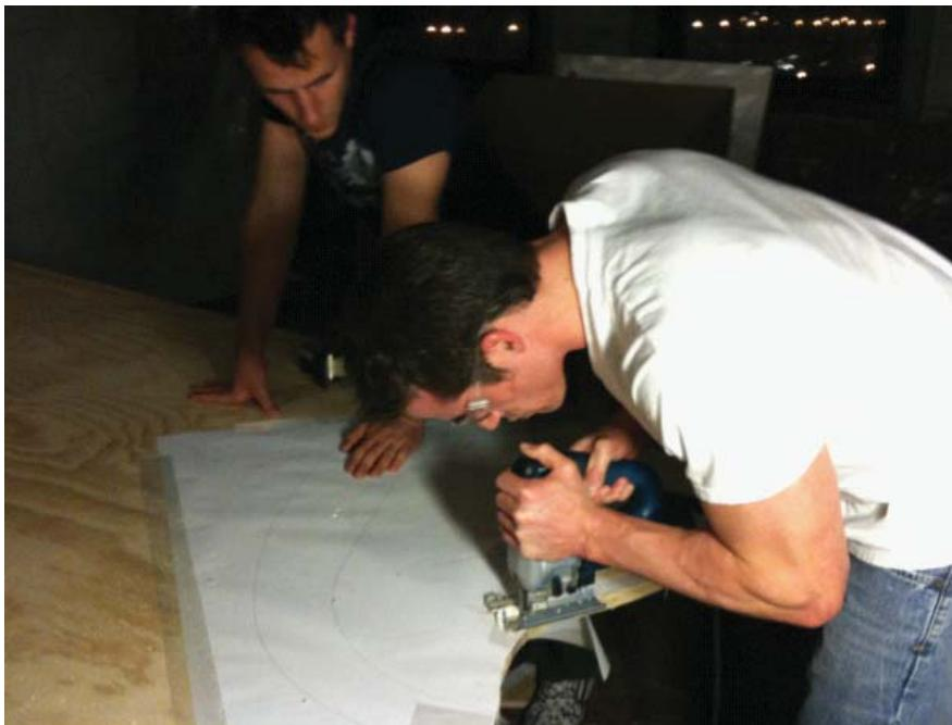
*cutting wind support discs with plotted template*
